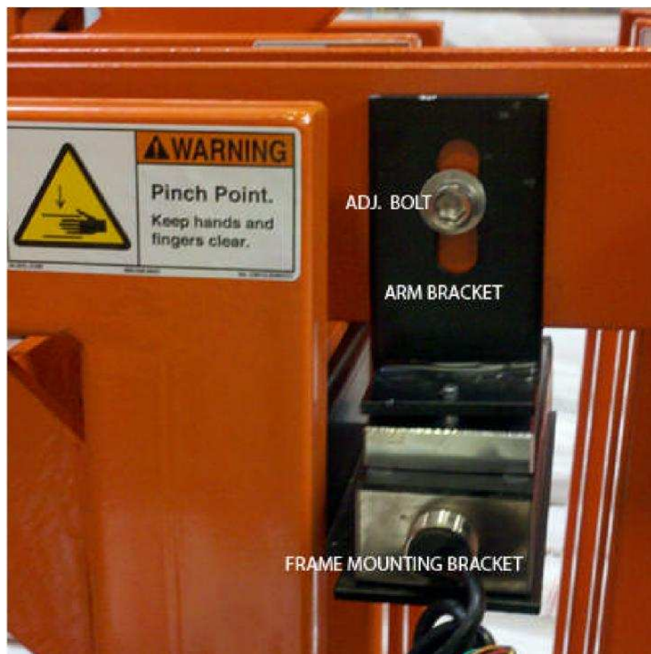
Pictured above is the magnet striker plate assembly for the arm-down magnetic lock .
